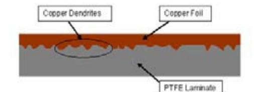
Figure 1 - Illustration of copper laminated to PTFE surface
