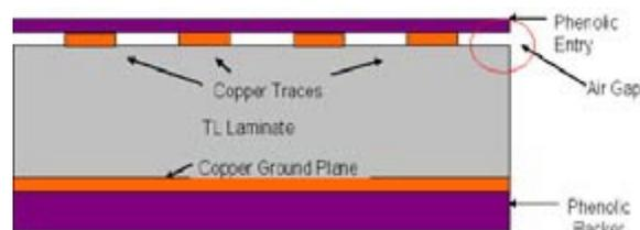
Figure 5 - A typical rout stack
