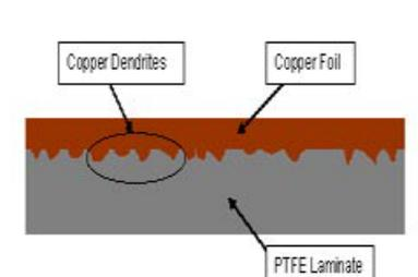
Figure 2 - Illustration of copper laminated to PTFE surface
