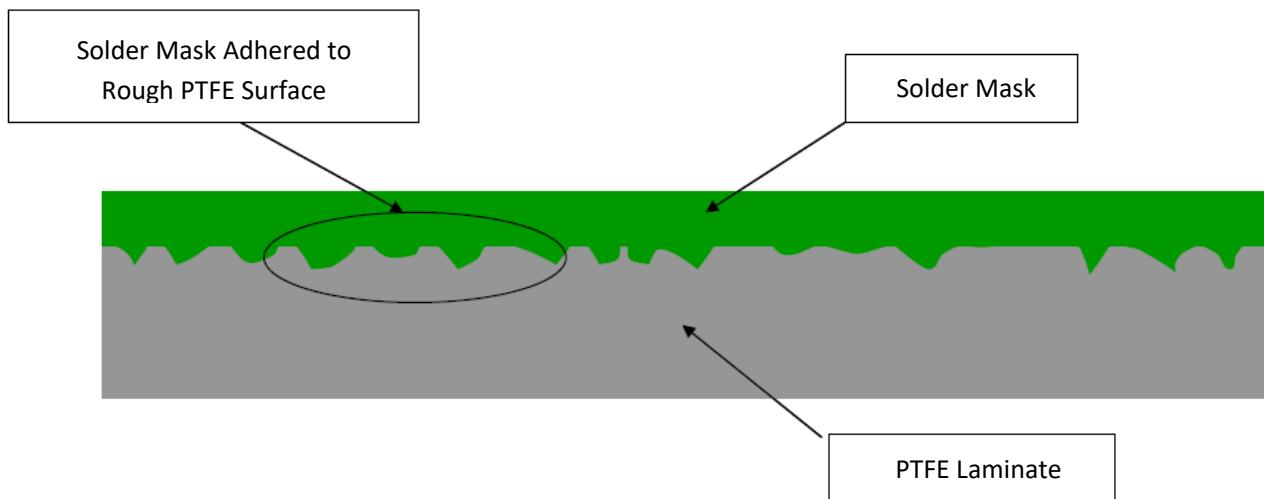
With the need to replace the process a substitute process has been used which has several added benefits. Chemical cleaning of the copper surface offers the advantage of reduced mechanical stress on the material. This becomes critically important when dealing with thin laminates (<0.010" or 0.25 mm) and/or critical dimensional tolerances in soldermask or second stage drilling or routing.
