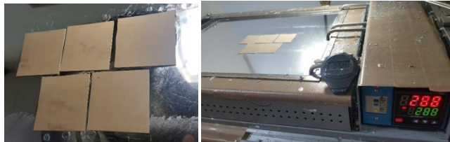
Fig. 14b: NF-30 during solder float at 288 °C
