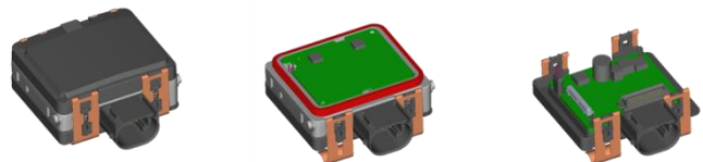
Fig. 3: 77 GHz ADAS Sensor (courtesy of Robert Bosch GmbH)
