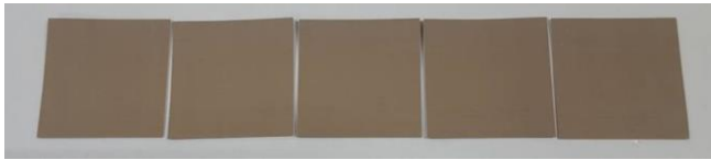
Fig. 14a: NF-30 before solder float at 288 °C
