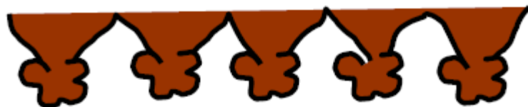
Standard ED copper foil treatment
